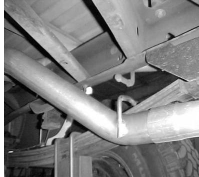
BOLT HEADPIPE #A USING SUPPLIED FLANGE GASKET #H AND REUSING FACTORY BOLTS. APPLY A SMALL AMOUNT OF HIGH-TEMP O2 SENSOR SAFE SILICONE ON THE FLANGE TO PREVENT ANY LEAKS. INSERT WELDED HANGER INTO RUBBER GROMMET. DO NOT TIGHTEN
